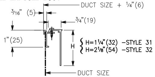
ED APPLICATION IS SUPPLIED COMPLETE WITH BORDER AND DUCT MOUNTING FRAME
