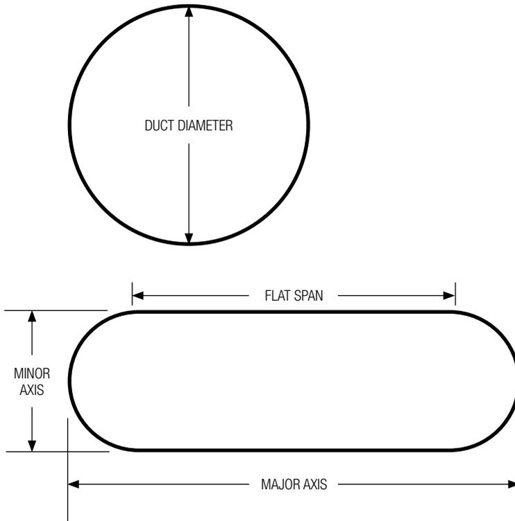
Example: If the height for the minor axis (round portion) is 10", the duct diameter for the spiral duct grilles is 10".
