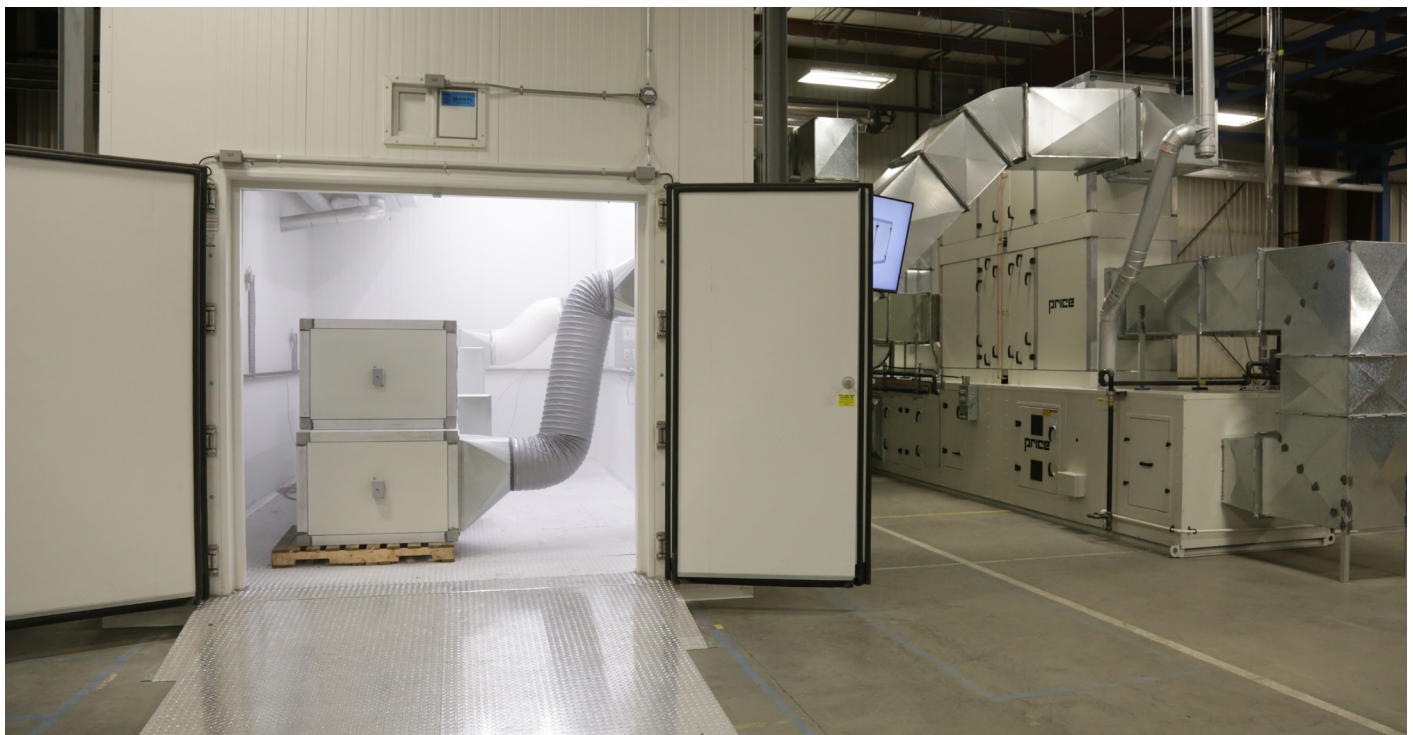
The Price Environmental Chamber is capable of testing products to meet ASHRAE 84, CSA C439, ISO 16494 and AHRI 1060 requirements while maintaining temperatures ranging from -40°C to +40°C (-40°F to +104°F)
