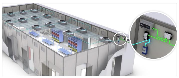
An example of Fan Filter Units in a cleanroom on a BACnet system. The BACnet router's MS/TP port links to the BACnet Commissioning Tool and the Fan Filter Units, and the Ethernet port connects to an IP switch that services the Web Server and the building's local area network (LAN).
